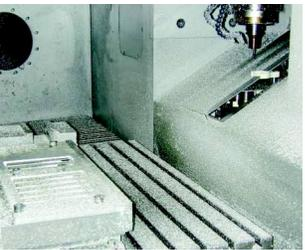
**To compensate for slight runout and the dimensional effects of a high rate of rotation, the machine uses non-contact tool setting to measure the tool's offsets at high speed. In this photo, the laser (which is not visible from this view) is located in the recess just below where the tool is positioned.**
